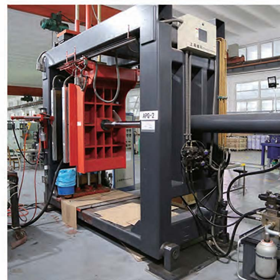
环氧树脂自动压力凝胶成型机 HAGV model APG shaping mill for epoxy resin machine
